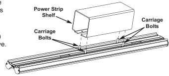
3. Thread four Nylon Wing Nuts onto each of the Carriage Bolts and tighten them when the Power Strip Shelf is in the desired position.
